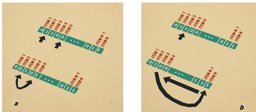
Figure 5. Construction of a neighboring solution. (a) The swap process to create a neighborhood solution; (b) shifting process to create a neighborhood solution.
