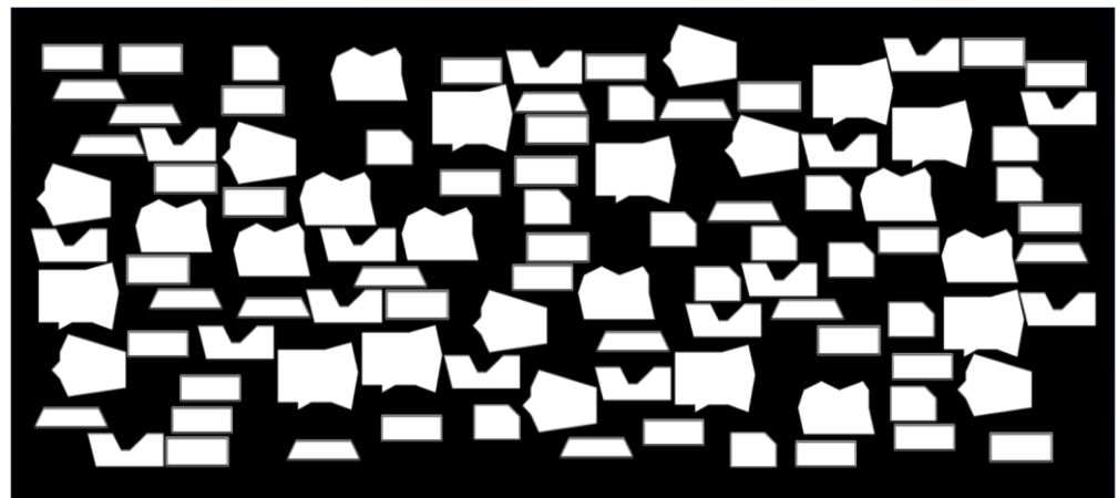
Figure 15. Solution found by the ILS algorithm inserting 101 pieces for the Shirts instance, consuming 2 h of processing time.
