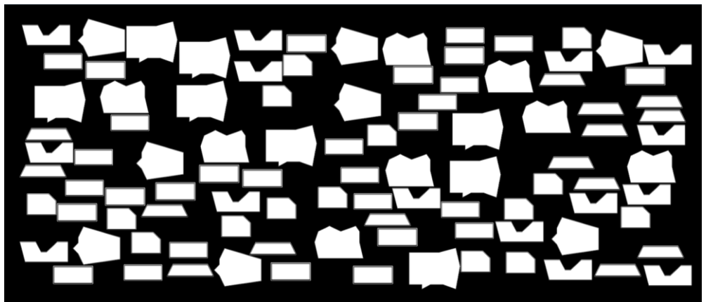
Figure 10. Solution found by the ILS algorithm using 99 pieces for the Shirts instance.
