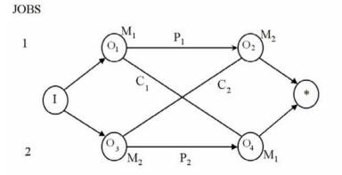
Fig. 1. Disjunctive Graph of the JSSP.
