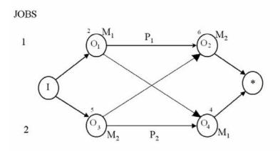
Fig. 4. JSSP instance with precedence restrictions.
