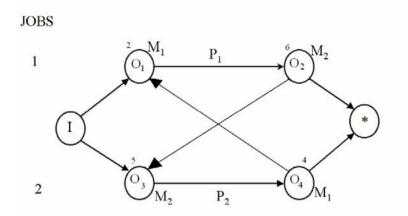
Fig. 5. JSSP instance with precedence restrictions.
